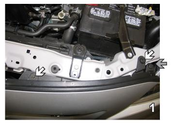
Using the Phillips screw driver, remove the Phillips screws (white arrow) from the top corner edge of the fascia. Remove push pin (gray arrow), do this to both sides and set aside for later reinstallation.
