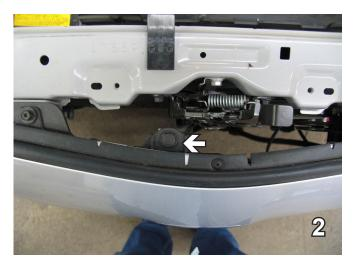
2. Remove push pin from top edge of fascia just below hood latch and set aside for reinstallation later.
