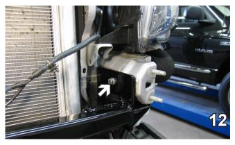
12. Insert 3/8"-16 x 1-1/4" hex bolts with 3/8" lock washers attached to 3/8"-16 nut plates with inserted into the frame rail on both sides to hold the baseplate in place.
