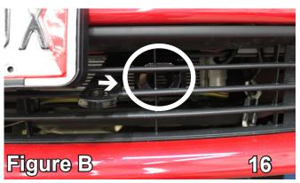
16. Hold the fascia as close to its original position as possible, mark and trim the grill with a utility knife to allow the baseplate receivers to come through. Reinstall the fascia.
