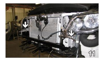
11. Slide the baseplate up between the frame rails, align with the existing hole on each side and clamp.
