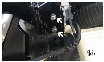
14. Insert 3/8"-16 x 1-1/4" hex bolts and 3/8" lock washers with 3/8"-16 nut plates with inserted into the frame rail. Use Loctite on all the bolts and tighten. Do this on both sides and the bolts inserted previously. Reinstall the bumper.
