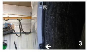
Just forward the front tire on the upper corner of the fascia and inside the wheel well, turn the screw 90° to remove it (white arrow). Using a flat screw driver, remove the upper push pin (gray arrow). Do this on both sides and set aside for later reinstallation.
