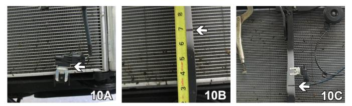
10. Move the bracket out of the way by sliding it up. Measure 7" up. Reroute the wire up and reattach the bracket so that the bottom of it is 7" up.
