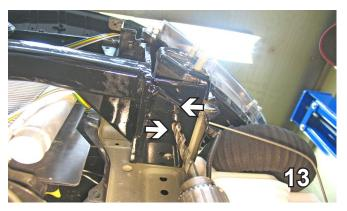
13. Using the baseplate as a template, drill both holes in the under side of the frame rail with a 13/32" drill bit. Do this on both sides.
